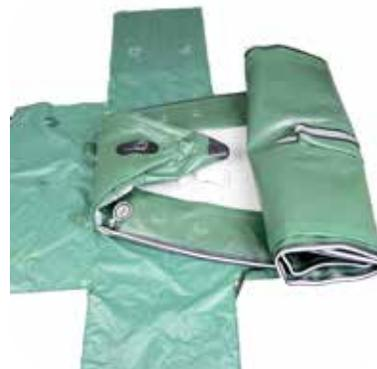
Keep folding toward the bow until the keel is visible. Make a crease between the logo and air valve and fold the tip back.
