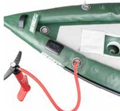
With valve stem in the up position, insert adapter, push down firmly and twist clockwise.
