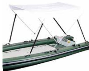
Attach the rear clips to the rear carry handles. Attach the front straps to either set of carry handles. Wrap the straps around the rod twice to use the handles directly below the strap. Adjust the straps until canopy is tight.
