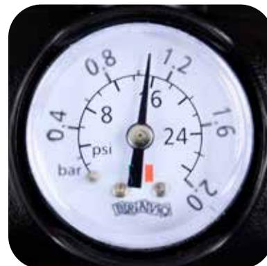
Pressure gauge will not register until chamber begins to get pressurized.
