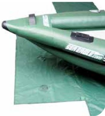
Spread boat bag on the ground. Pull boat over the bag so it overhangs edge of bag by about 4". Remove transom, seat frames, Scotty accessories (but not the screwed-in base), etc. Transom must be removed for boat to fit in bag.
