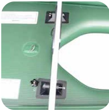
Starting with the floor grommets, insert bolts with flat washer through grommet and transom.
