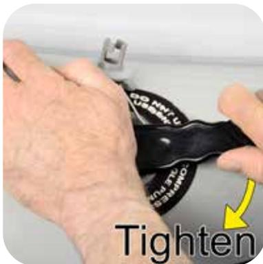
Press on center of valve tool with free hand to keep from breaking the teeth off the tool. If loosening a very tight valve, an extension tube might be needed.
