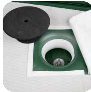
**⚠ Caution:** Avoid falls. Always place the plug into the keel valve access hole. Stepping onto the unsupported cover could cause injury.
