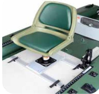
Assemble and install the Swivel Seat Frame. This is a one-time assembly. The assembled frame can be removed for deflation and folding the boat.
