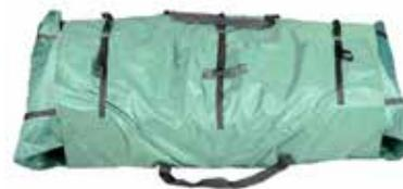
Secure the bag with the straps. Run strap through both rings, and back through first ring. Pull tight. Folded dimensions are approximately 58 x 27 x 13". To avoid damage, do not drag the folded boat.
