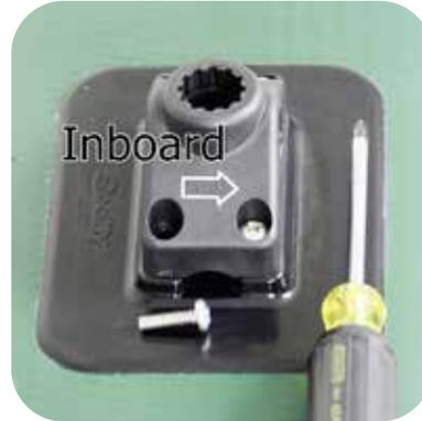
Use the 7/8" screws to secure the mounting base to the pad. Orient the base so arrow points inboard.
