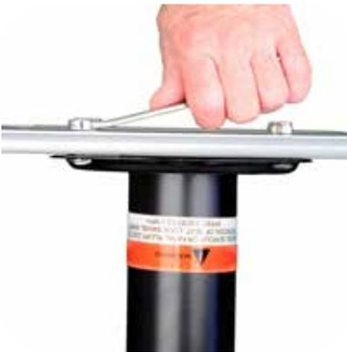
Attach pedestal to aluminum board using the 1" hex head bolts and locking nuts.
