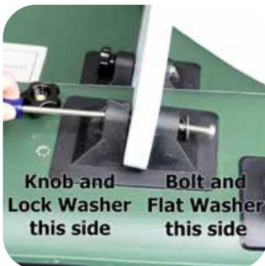
If needed, use a screwdriver to move the grommet to the hole. When all four bolts are inserted, put the lock washers on and secure with the knobs. If needed, hold the nut head with a wrench and tighten the knobs. Inflate the side chambers to working pressure.
