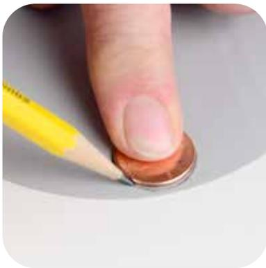
Trace the outline of a penny on the patch material and on the boat. If a larger patch is needed, use a larger item as a template.
