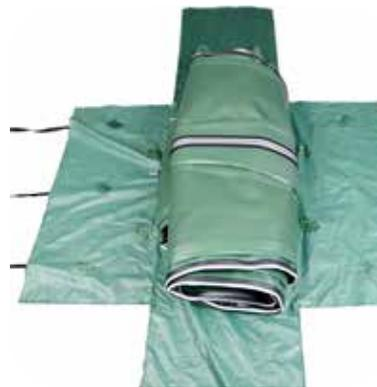
Fold the boat onto the bow. If the boat came with a strap, wrap the clip the strap around the boat.
