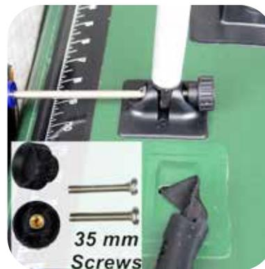
Place canopy on back of boat with short bars up. Canopy frame is wider than boat, push rods inward. Use the 35mm screw and knob to secure rod to canopy mounting pad. *Note:* This step is easier when the side rods are vertical.
